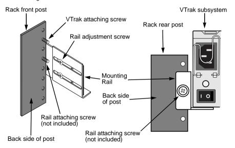
Figure 2. Mounting rail installation
